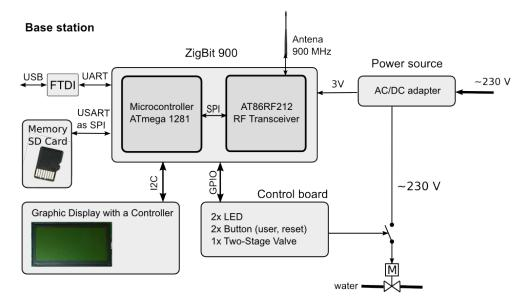
Figure 2: Block diagram of the base station
