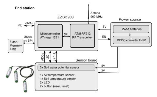
Figure 1: Block diagram of end station
